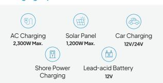
Note: Shore power charging: An extra adapter cable is required. How to connect: shore power outlet  $\rightarrow$  adapter cable  $\rightarrow$  charging inlet of AC240P.
